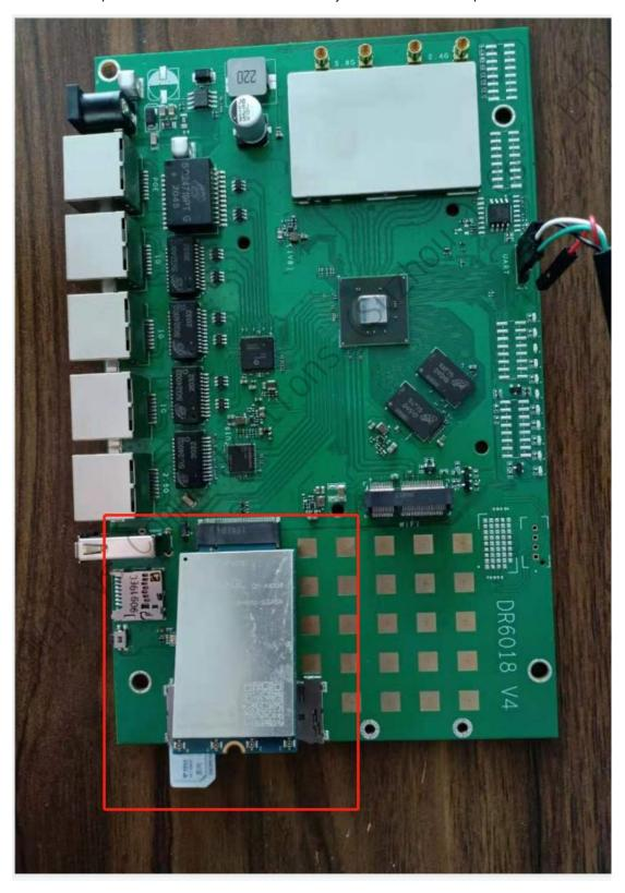
2. Connect the board by UART localhost and login: root, Password: asdf1234
